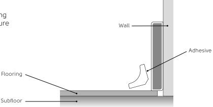
Use finishing nails every 450mm (16") through the scotia into the skirting. Be sure to pre-drill any holes.
